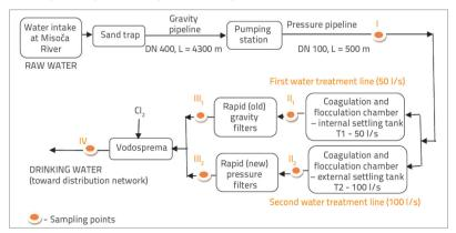
Figure 1. Block diagram of the water treatment technology at the water supply system in Ilijaš municipality
