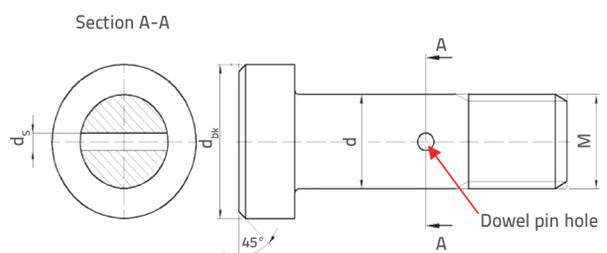
Figure 6. Typical bolt scheme [9]
