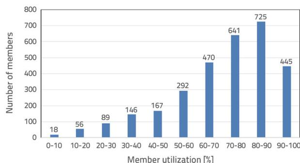
Figure 8. Member utilization histogram of a fully designed structure [7]
