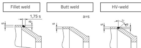
Figure 4. Cone-tube weld types [9]
