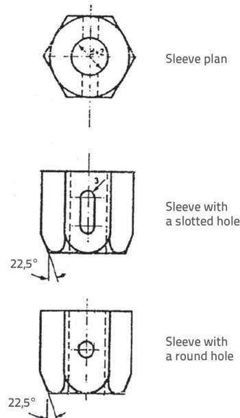
Figure 5. Hexagonal sleeve types [10]
