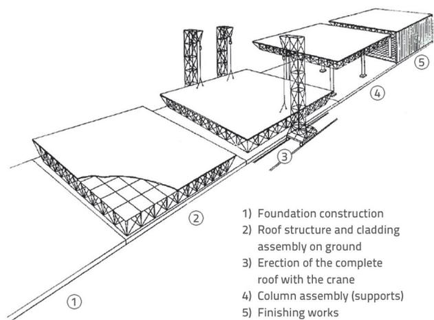
Figure 12. Segmental method's order of operations [8]
