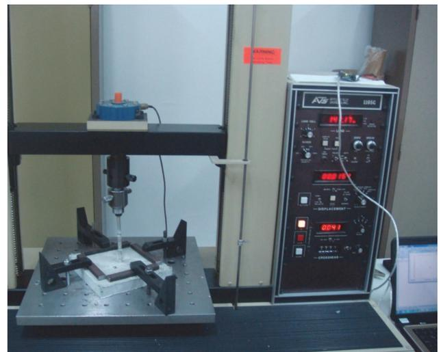
Figure 12. Tensile testing of the embedded anchorage element
