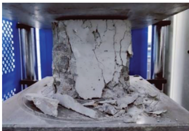
Figure 2. Failure pattern of concrete standard test block
