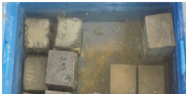
Figure 4. Cube specimens immersed in water
