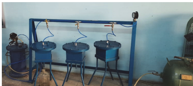
Figure 5. Water permeability test apparatus
