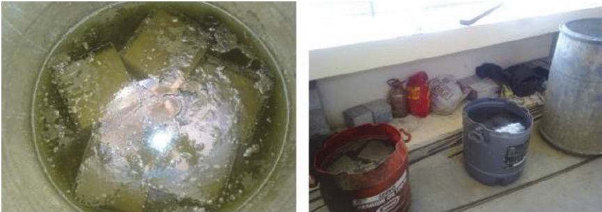
Figure 3. Cube specimens immersed in HCl solution
