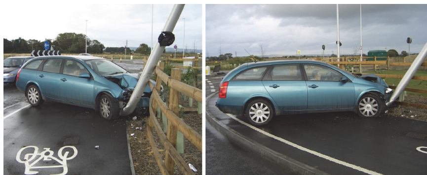
Figure 3. Vehicle collision with a passively safe pole [9]
