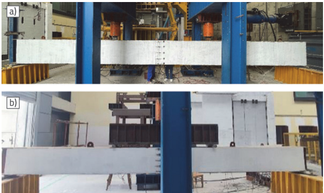
Figure 9. Specimen loading diagram: a) Loading device of PECB1, PECB3 and PECB5; b) Loading device of PECB2 and PECB4
