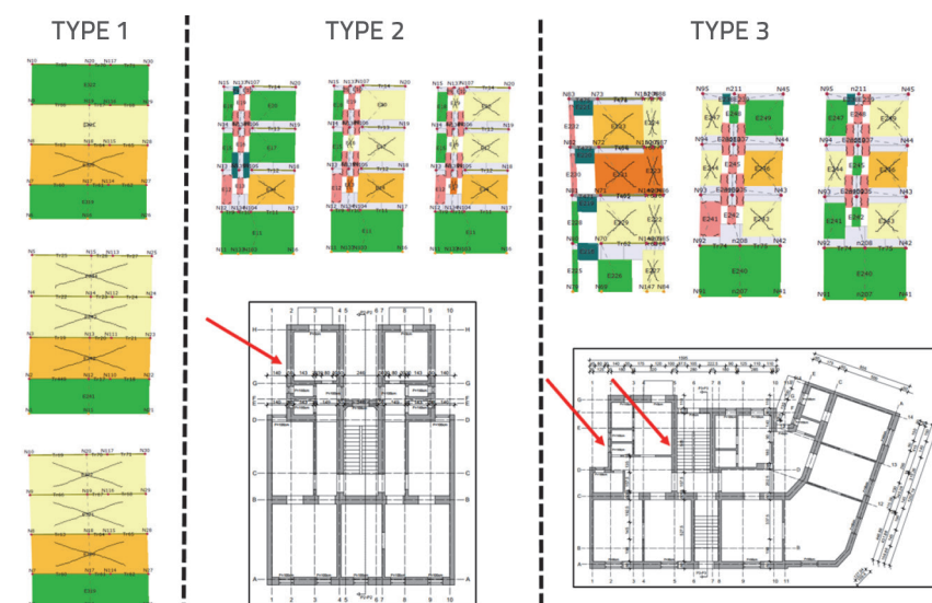
Figure 29. Critical positions for the three structural types in the original and strengthened states
