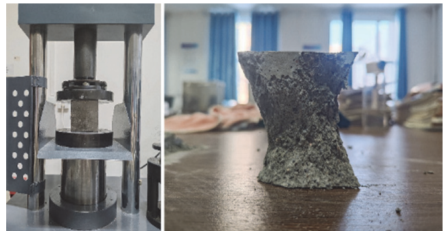
Figure 5. Failure morphology of DSBFC under compressive loading
