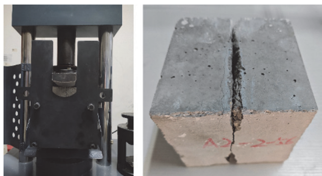
Figure 7. Splitting tensile strength failure morphology of DSBFC
