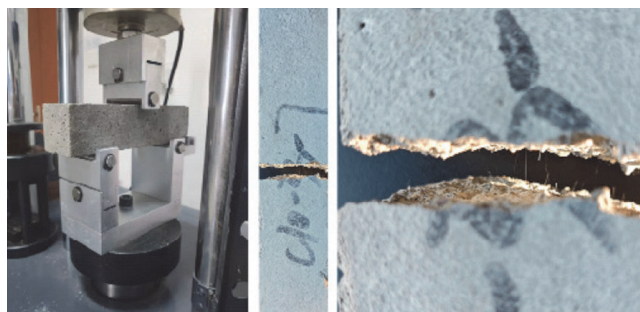
Figure 6. Flexural strength failure morphology of DSBFC
